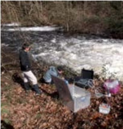
Measuring CO<sub>2</sub> partial pressure in the Leyre's water – CNP Leyre project
